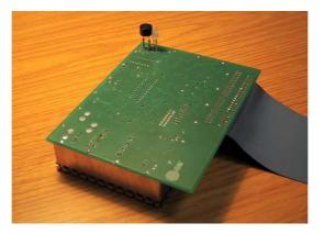
Figure 4: Receiver used to detect ultrasonic signals.
