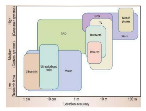
Figure 1: a diagram shows the range of accuracy of each usable technology, where the top boundary technologies shows the new and next generation of current technologies. [30]
