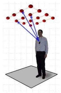
Figure 3: How triangulation works with Active Bat [11]
