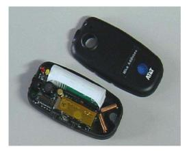
Figure 5: AT&T developed Active Bat sensor http://www.cl.cam.ac.uk/research/dtg/attarchive/bat/flatBatInside.jpg
