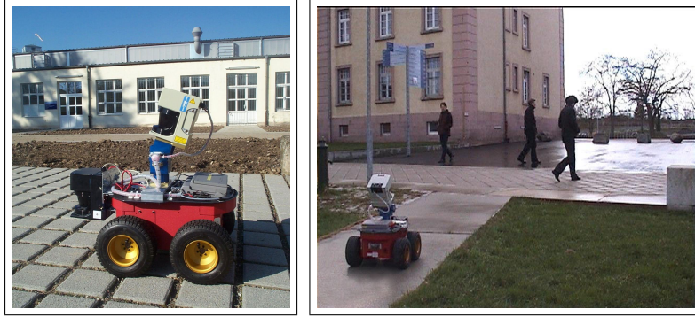
Figure 13. Pioneer 2 AT robot Herbert for 3d outdoor mapping (left) and typical situation in which people walk through the scene during mapping (right).
