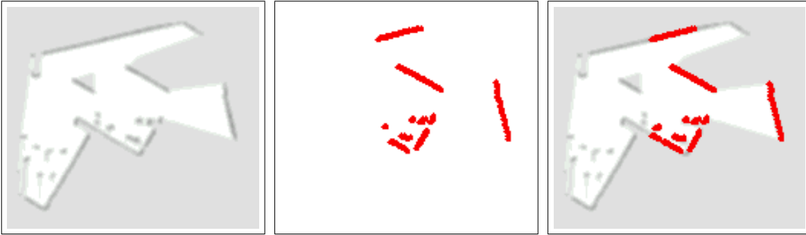
Figure 4. Two-dimensional scan alignment: Map created so far (left image), measurement s_t obtained at time t (center image) and resulting alignment (right image).
