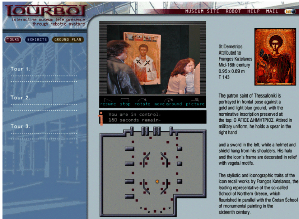
Figure 11. Web interface of the TOURBOT system for exclusive control over the robot.
