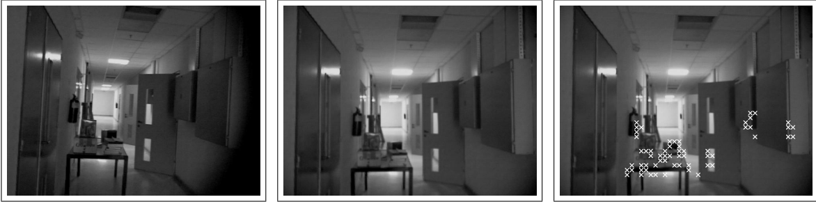
Figure 3. Images captured at time t - 1 (left image) and time t (center image) and results of the evaluation process projected on the image captured at time t (right image).
