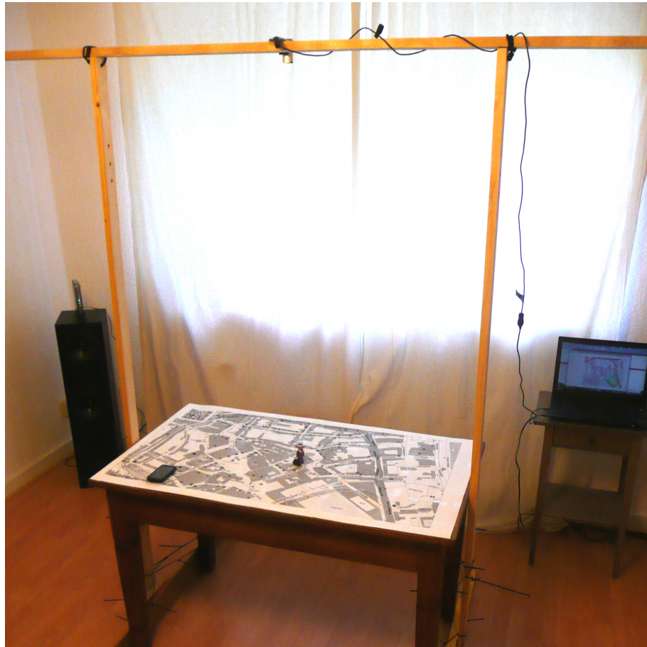
Figure 1.1: The hardware setup of the Presence Simulator - A system developed in this thesis to simulate and track the user's presence in a model landscape.
