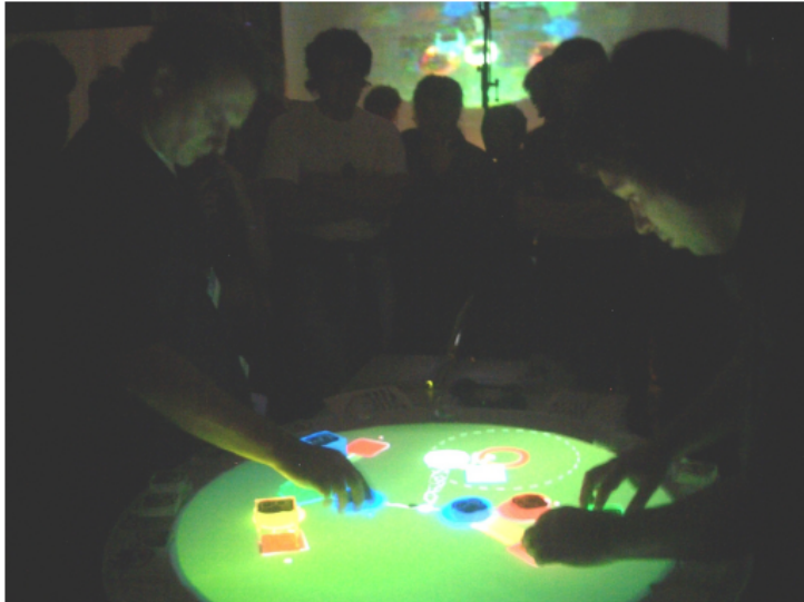
Figure 2.1: reactTable is a digital musical instrument and an application of the reactIVision project. Fiducial markers at the bottom of the objects on the table are tracked by a camera underneath the table. [rea05].
