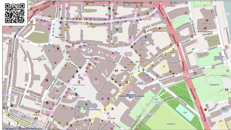
Figure 3.8: Map area saved in a PDF file for later use. The openstreetmap map provider is used here. Map position, scale and orientation are encoded in a QR Code which is used by the Presence Simulator's auto calibration system.
